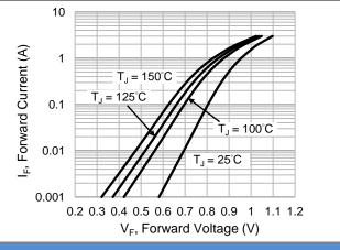
Fig.4 Typical Forward Characteristics
