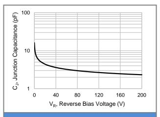
Fig.2 Typical Junction Capacitance
