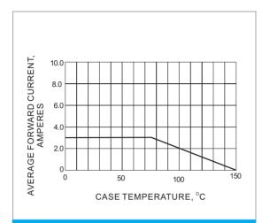
Fig.1-FORWARD CURRENT DERATING CURVE
