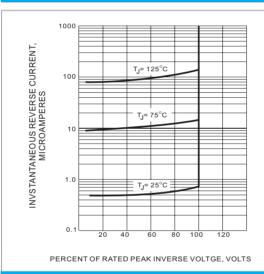
Fig.3-TYPICAL REVERSE CHARACTERISTICS
