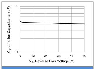
**Fig.2 Typical Junction Capacitance**
