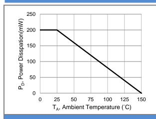
**Fig.1 Power Derating Curve**
