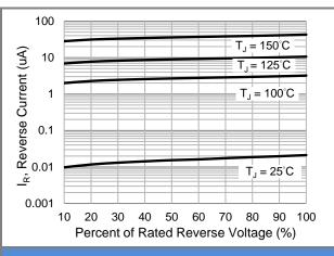
Fig.3 Typical Reverse Characteristics
