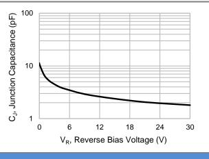
Fig.2 Typical Junction Capacitance
