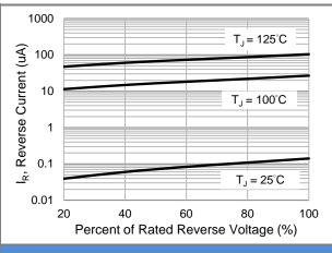
Fig.3 Typical Reverse Characteristics
