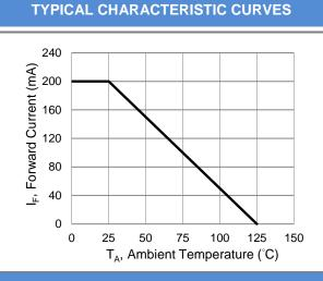
Fig.1 Forward Current Derating Curve
