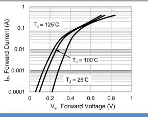
**Fig.4 Typical Forward Characteristics**
