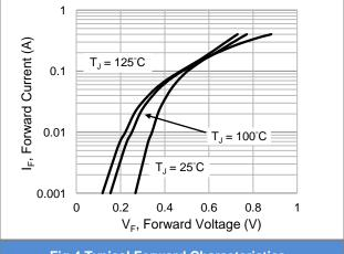
Fig.4 Typical Forward Characteristics
