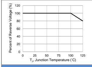
Fig.5 Operating Temperature Derating Curve
