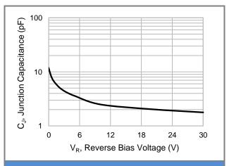
**Fig.2 Typical Junction Capacitance**
