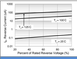
Fig.3 Typical Reverse Characteristics
