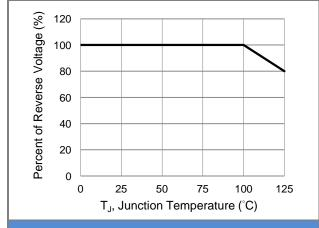
Fig.5 Operating Temperature Derating Curve
