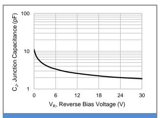
**Fig.2 Typical Junction Capacitance**
