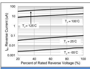
Fig.3 Typical Reverse Characteristics
