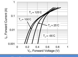
Fig.4 Typical Forward Characteristics
