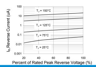
Fig.3 Typical Reverse Characteristics
