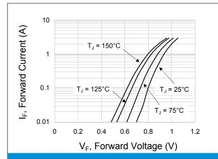
Fig.4 Typical Forward Characteristics
