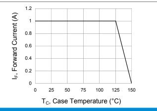
**Fig.1 Forward Current Derating Curve**
