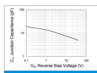
Fig.2 Typical Junction Capacitance
