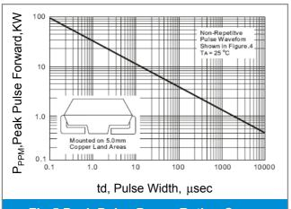
Fig.5 Peak Pulse Power Rating Curve
