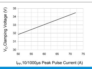
Fig.3 Typical Peak Clamping Voltage
