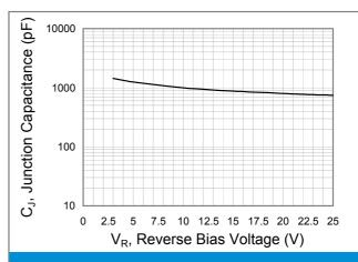
**Fig.2 Typical Junction Capacitance**
