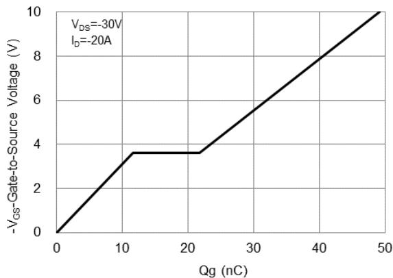
Fig.7 Gate-Charge Characteristics
