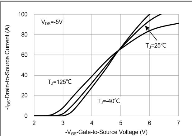
Fig.2 Transfer Characteristics
