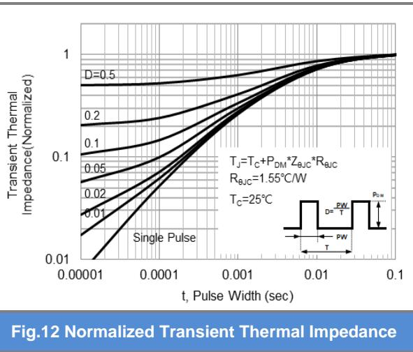
Fig.12 Normalized Transient Thermal Impedance
