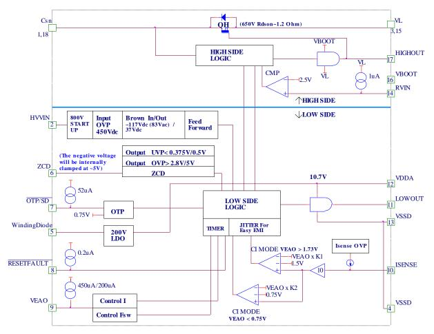
Note: Q<sub>H</sub>: 650V/4A SJMOS, R<sub>DS(on)</sub> typ.=1.2Ω
