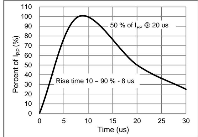
Fig.2 Pulse Waveform
