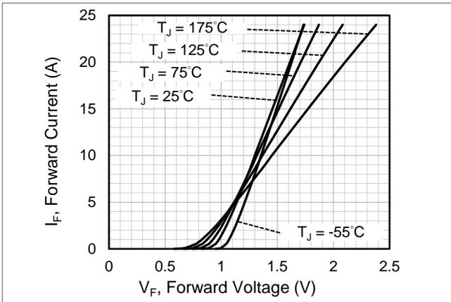
Fig.1 Forward Characteristics
