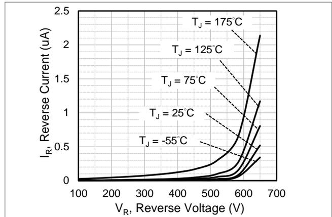
Fig.2 Reverse Characteristics
