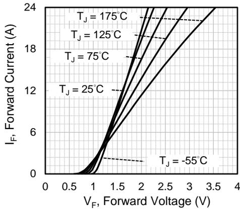
Fig.1 Forward Characteristics
