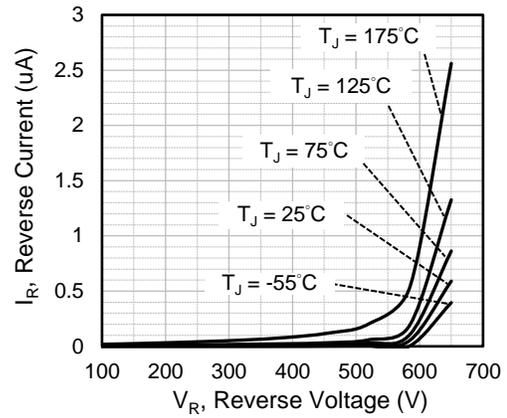
Fig.2 Reverse Characteristics
