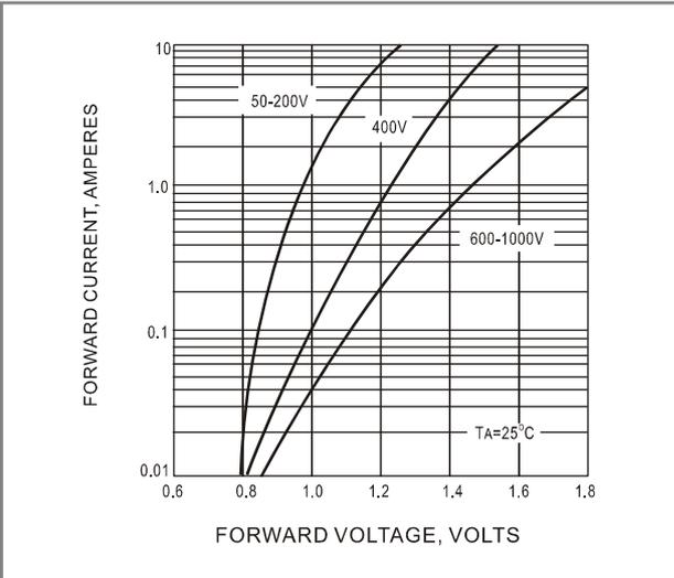
**Fig.3 FORWARD CHARACTERISTICS**
