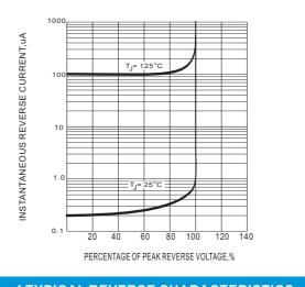
Fig.4 TYPICAL REVERSE CHARACTERISTICS
