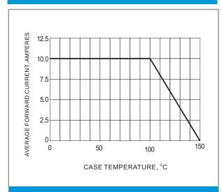
Fig.1 FORWARD CURRENT DERATING CURVE
