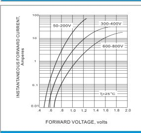
Fig.3 FORWARD CHARACTERISTICS
