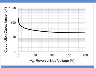
**Fig.2 Typical Junction Capacitance**
