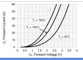
**Fig.4 Typical Forward Characteristics**
