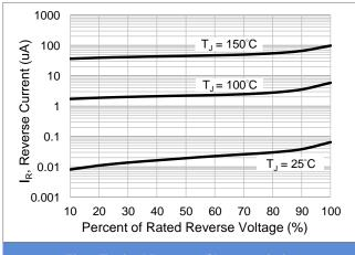
Fig.3 Typical Reverse Characteristics
