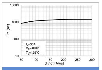
Fig.6 Typical Reverse Recovery Charges Versus di/dt
