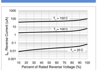
Fig.3 Typical Reverse Characteristics
