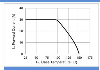
**Fig.1 Forward Current Derating Curve**
