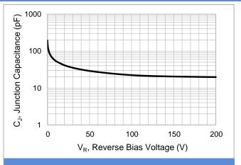
Fig.2 Typical Junction Capacitance
