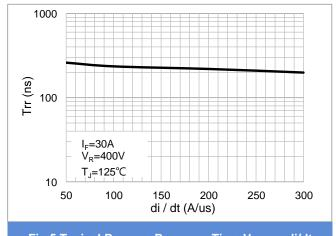
Fig.5 Typical Reverse Recovery Time Versus di/dt
