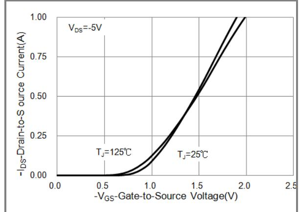
Fig.2 Transfer Characteristics
