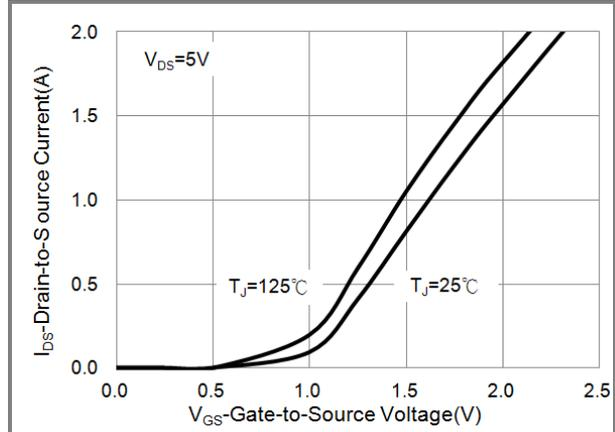
Fig.2 Transfer Characteristics
