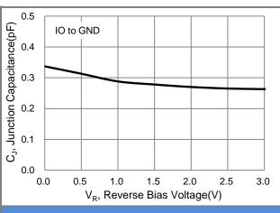
Fig.3 Typical Junction Capacitance
