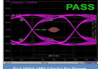
Fig.6 10Gb/s USB3.2 Gen2x1 Eye Diagram
