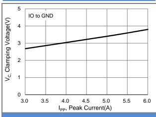
Fig.1 Typical Peak Clamping Voltage
