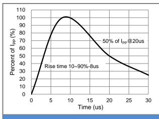
Fig.2 Pulse Waveform
