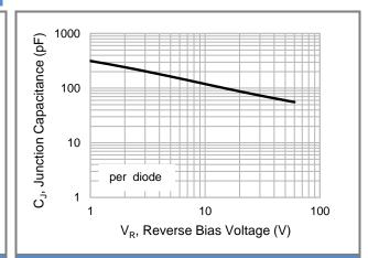
**Fig.2 Typical Reverse Characteristics**
