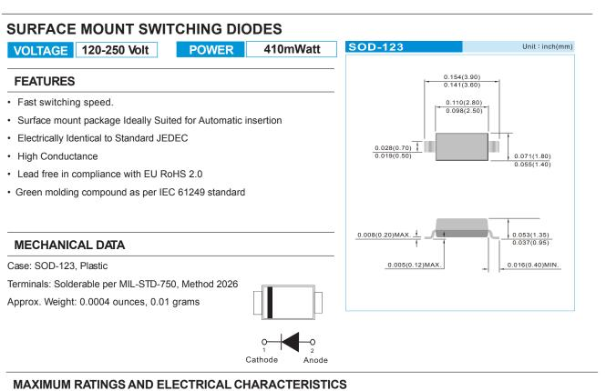
Ratings at 25°C ambient temperature unless otherwise specified. For capacitive load, derate current by 20%.
