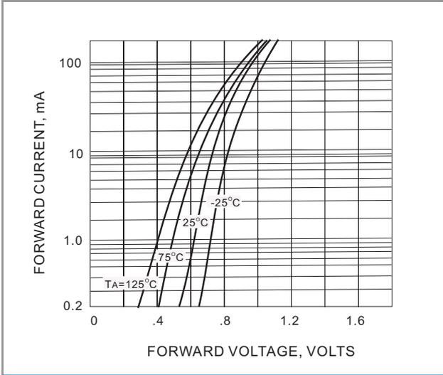
Fig.1 FORWARD CHARACTERISTICS
