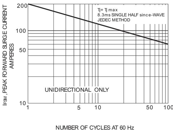
**Fig.5 MAXIMUM NON-REPETITIVE PEAK FORWARD SURGE CURRENT UNIDIRECTIONAL**
